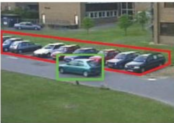
FIGURE b) Object tracking is to distinguish the object of interest (green) from clutter in the background (red).
