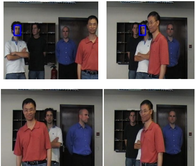
FIGURE2.2:- Tracking is possible as long as the selected object is visible in the image. In the third frame an occlusion occurs.
